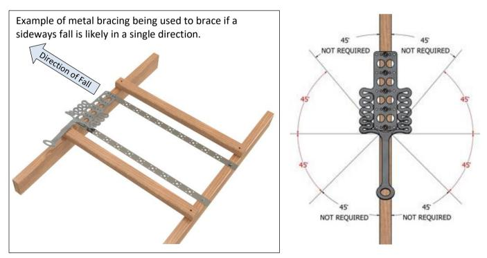
For TileLinks installed on structure under 45mm x 90mm MGP10 pine or equivalent, which can be loaded sideways suitable bracing must be installed to support the structure if not assessed as adequate.
