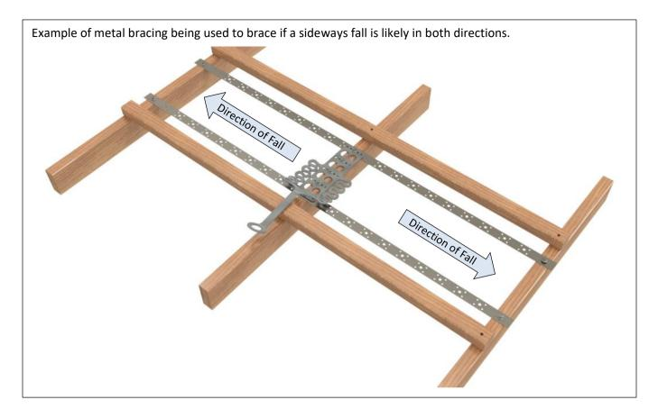
Bracing may be required for sideways loads due to rafter size, location of rafter (high in the hip) and existing additional structural bracing (existing batten locations, noggins, metal bracing, plywood decking). Assessment will always need to be made by a competent person for each anchor installation at time of install.
